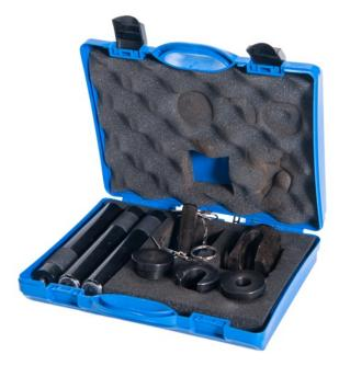
The extractometer is a control tool to check the traction resistance of the plugs.
